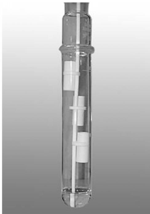
Fig. 1. PTFE cups arranged on a PTFE stick: outside and inside the glass reaction vessel.
