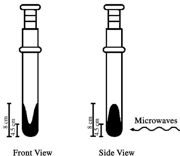
Fig. 2. Schematic of microwave radiation distribution inside the reaction vessel.
