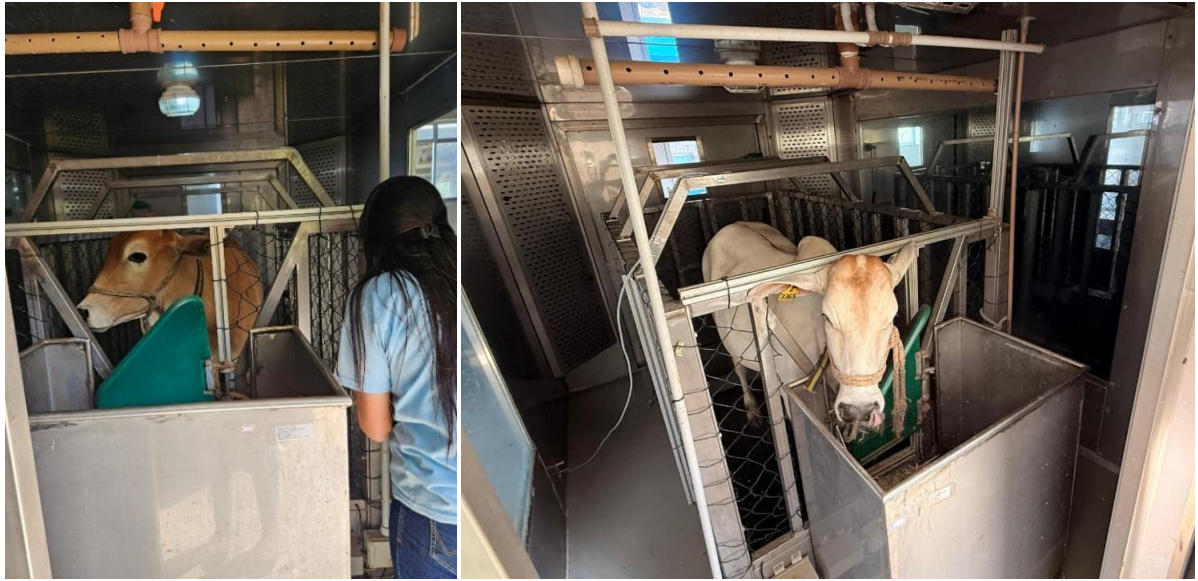
Figure 4. Measurements of methane production in the respiration chamber.
