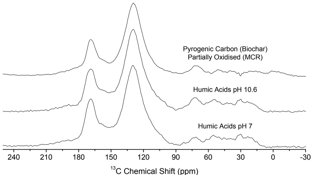
**Figure 1.** Solid State  $^{13}\text{C}$  NMR of the characteristic humic fraction from *Terra Preta de Índios* and the simulated spectra obtained by MCR.
