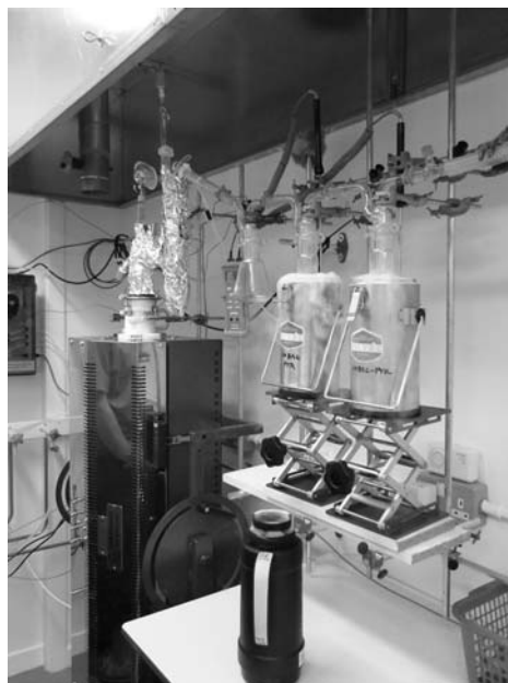
Figure 1. Batch lab-scale pyrolysis unit for biochar production at the UKBRC pyrolysis lab.
