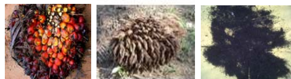
Figure 3. a) Palm Oil fruit bunch b) Empty fruit bunch (EFB) c) EFB biochar
