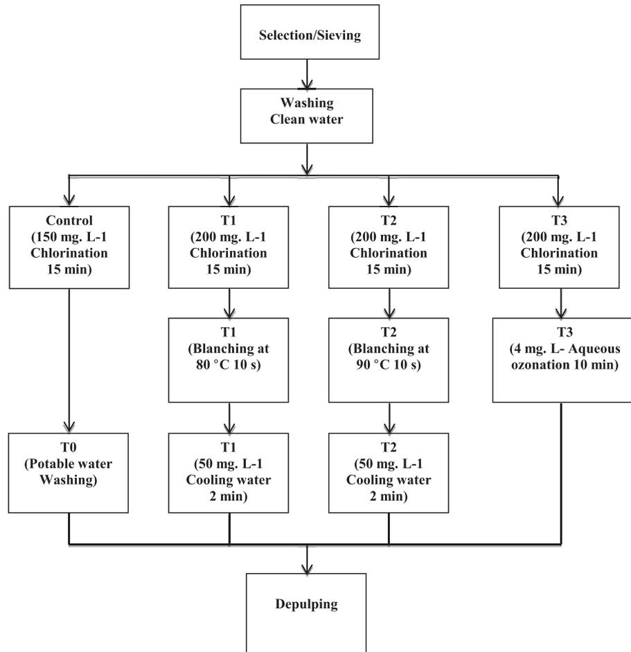
**FIG. 1.** FLOW DIAGRAM OF PROCESSING AÇAÍ FRUITS IN THERMAL AND NONTHERMAL TREATMENTS
