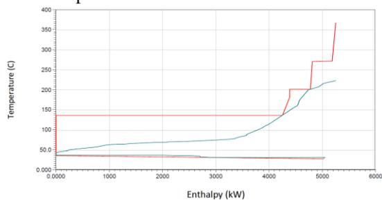
Figure 4 shows the grand composite curve of the integrated biodiesel and bioethanol plant with data presented in Table 4. The potential of 26.5% and 44.8% reductions in heating and cooling utilities, respectively, can be observed in the integrated plants when compared to the two stand-alone plants.
