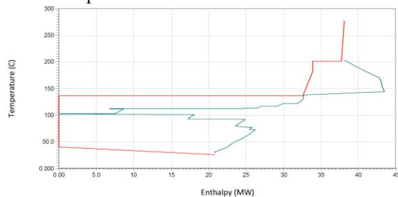
**Figure 3.** Utility integrated grand composite curve of biodiesel plant.
