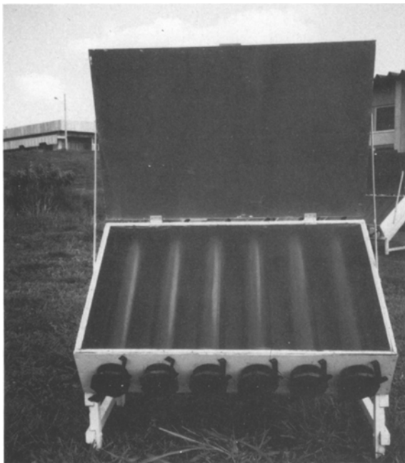
Fig. 1. Solar collector with tubes of 15 cm diameter and aluminium lid positioned to reflect the sun to the tubes filled with infested soil.
