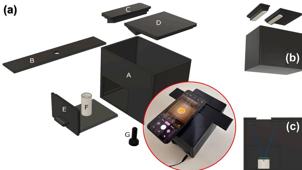
Fig. 1. (a) Exploded view of the box, showing the main body (A), adjustable slit for mobile camera (B), short and long lids (C and D), both with angled supports for LED strips), sample tray (E), sample holder (F) and sample compactor (G). Details of the (b) disposition of the LED strips under the angled lids (white blocks) and (c) representation of the light beams (blue lines). A photograph of the smartphone camera integrated into the analytical system, capturing an image of a coffee sample, is presented in the red inset.
