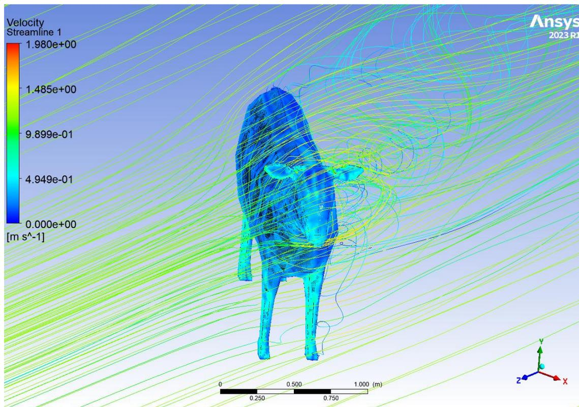
**Figure 4** Treelines from CFD simulation for dairy cattle orientation at 45°.
