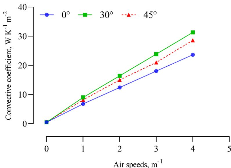
**Figure 1** Comparison of the convective heat transfer coefficient on different dairy cattle orientations.
