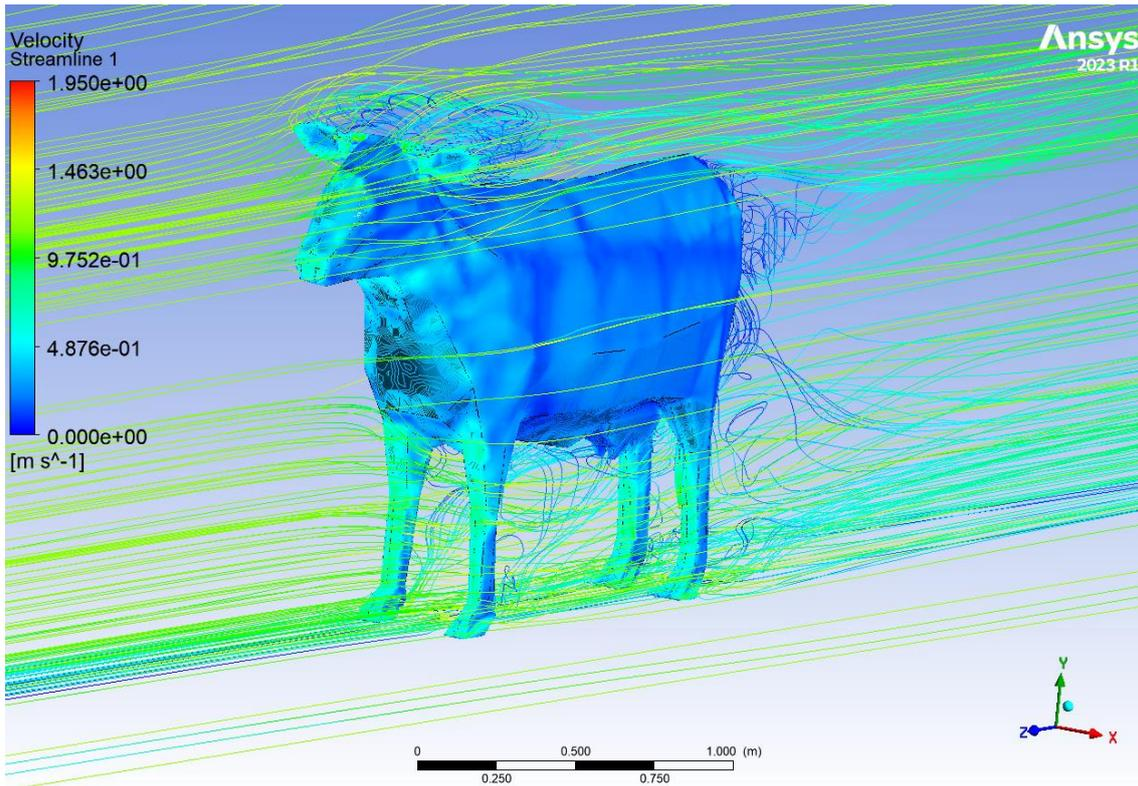
Figure 2 Tremlines from CFD simulation for dairy cattle orientation at 0°.
