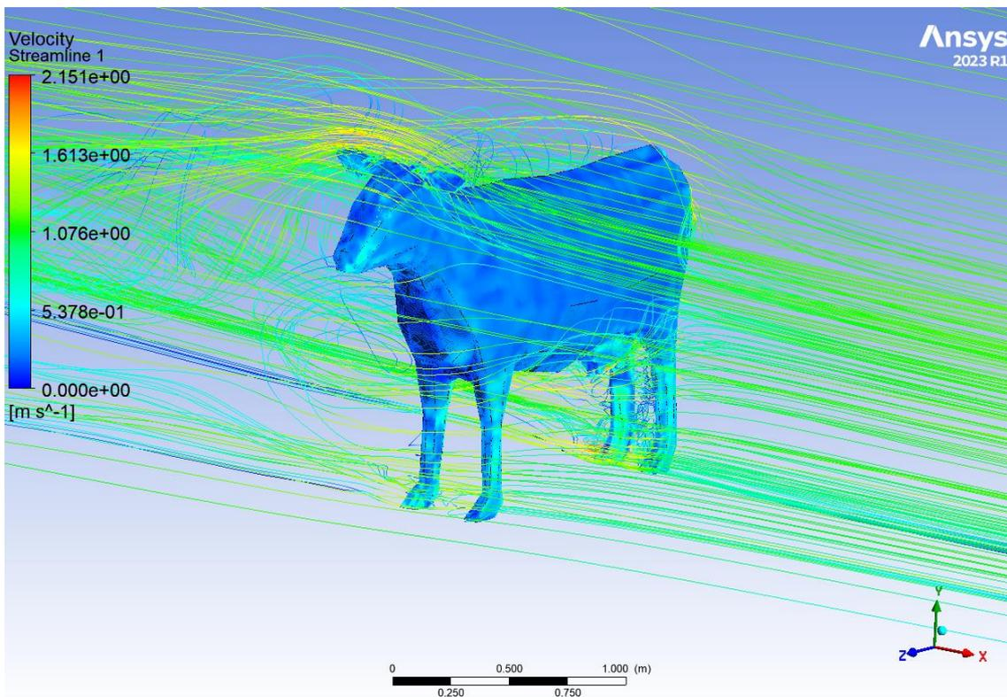
Figure 3 Tremlines from CFD simulation for dairy cattle orientation at 30°.
