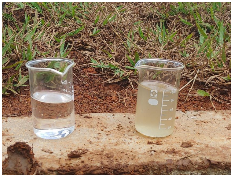
Figure 6 – Image of the effluent sample collected in the Septic Tank (right) and the reuse water (left) produced by the ReAqua System.
