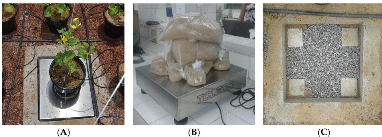
Figure 1. Weighing lysimeter installed in the experimental area (A), calibration of the weighing platform (B), and positioning in the experimental field on a masonry base (C).
