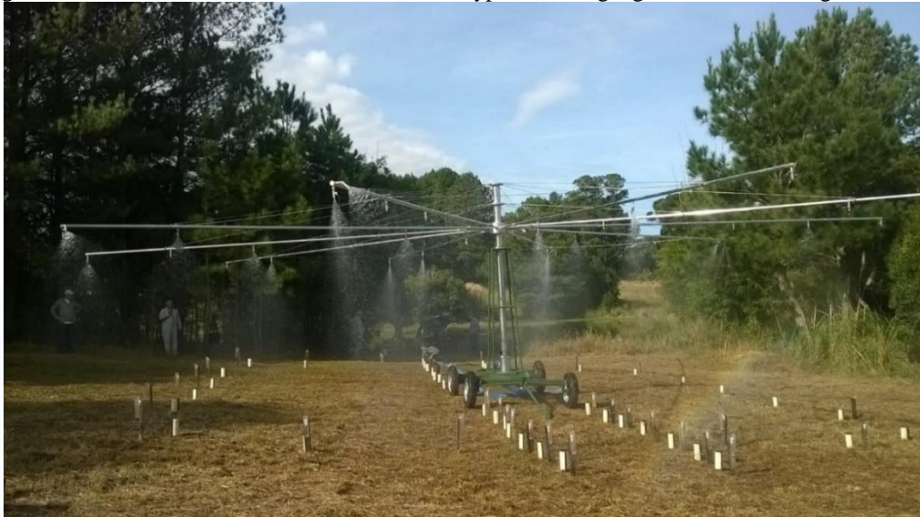
Figure 1: Overview of the rainfall simulator thrust type and rain gauges installed above ground level.
