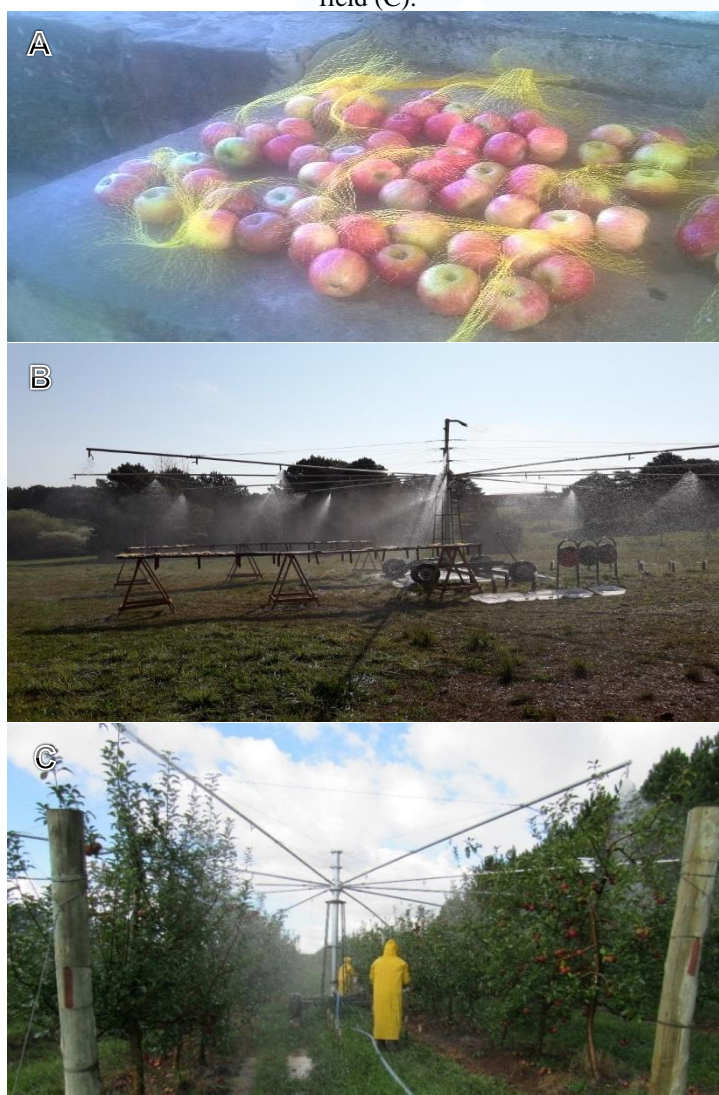
Figure 4: Apples packed in net-type fruit bags for dipping in the insecticide solution (perfect application) (A). Rainfall produced by the push-type rainfall simulator on the benches with treated apples in the perfect application test (B). Rainfall produced by the push-type rainfall simulator on apple trees in the field (C).
