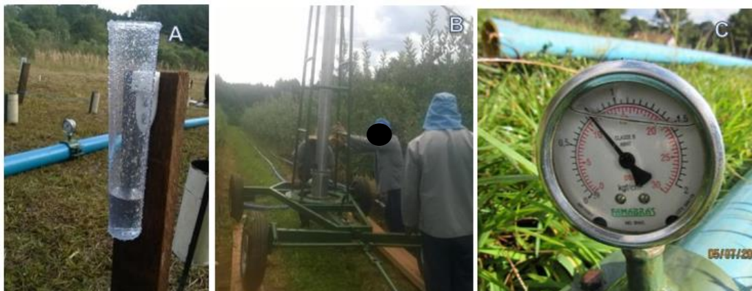
Figure 3: Rain gauge used to measure rainfall (A), rainfall simulator leveled with planks and wooden blocks (B), and pressure gauge to check system pressure (C).
