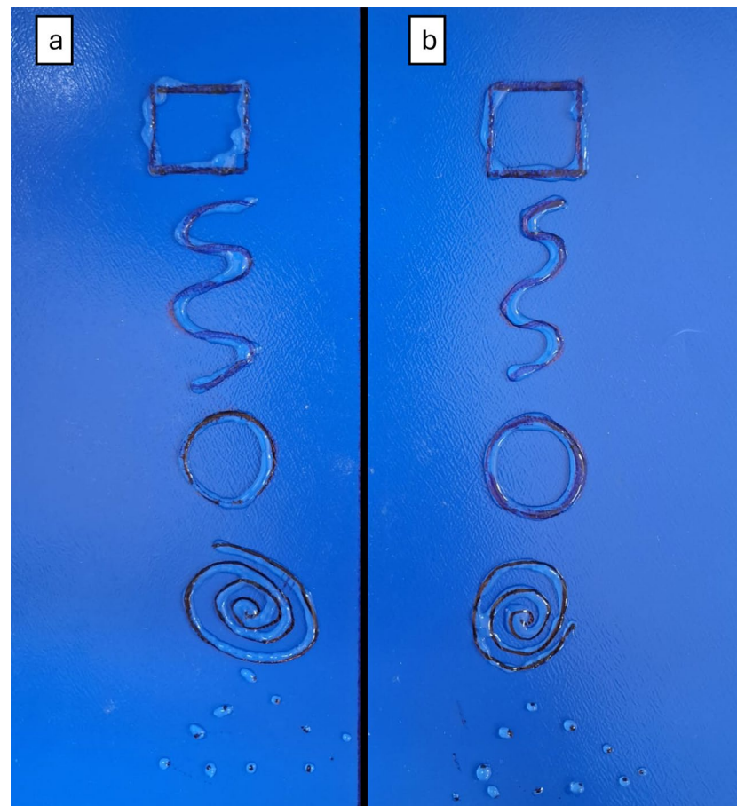
Figure 7. Manually extruded hydrogels in different forms and shapes. (a) Hydrogel 6; (b) hydrogel 14.
