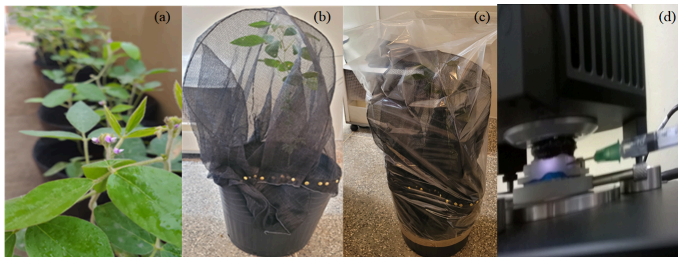
Figure 2. Soybean plants (a) with annealed wire frames and nylon shade cloth (b), sealed containers with the plastic film (c), and injection of volatiles into the gas chamber (d).
