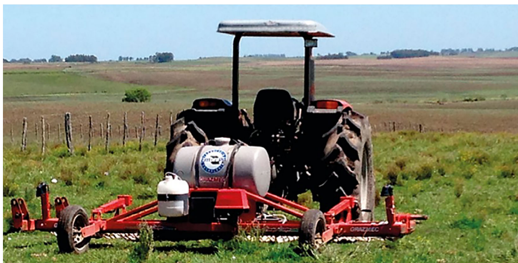
FIGURE 6 Selective glyphosate wiper applicator (Campo Limpo ® ) for Eragrostis plana control (Perez, 2015).
