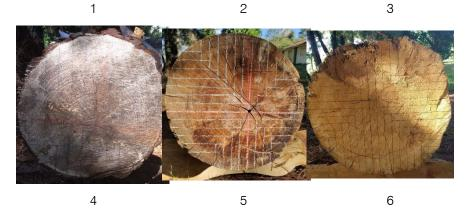
*Fig.* 15: Designed sections of Logs 1–6 with pieces of thickness 32 mm (27 + 5 mm) and width > = 50 mm and marrow bias of 2 cm (log 1); 4 cm (log 2); 4.5 cm (log 3); 5.3 cm (log 4); 6 cm (log 5) and 6.5 cm (log 6)
