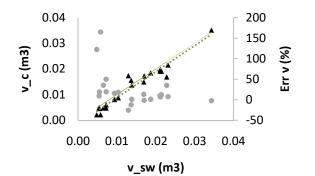
*Fig. 9:* Scattering between the calculated lumber volume ( $v_c$ ), the observed lumber volume ( $v_sw$ ), and accuracy (*Err* v)
