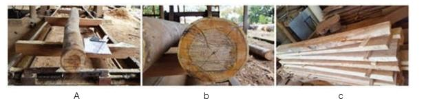
*Fig. 4:* a) Log in the sawmill machine, b) smaller face of a log with pieces calculated and selected to be cut, and c) stacked pieces to dry after measurement and identification
