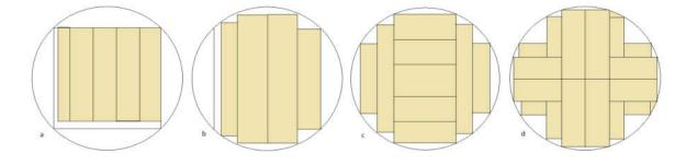
Fig. 1: Cut patterns for milled wood: a) circumscribed square; b) longitudinal; c) 180° 90° turn log; and d) radial
