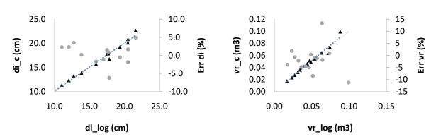
*Fig.* 7: a) Scattering between the observed diameter withbark ( $di\_log$ ) and the calculated diameter with bark ( $di\_c$ ) and its accuracy (*Err di*), and; b) scattering between the log volume ( $vr\_log$ ) and the calculated log volume ( $vr\_c$ ) and its accuracy (*Err vr*)
