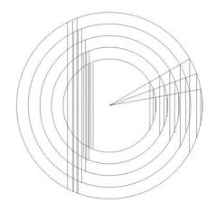
*Fig. 3:* Slab angles of 10, 20, and  $30^{\circ}$ , which show variable slab widths (right side of the circle) and chords defined by radius ratios of 0.55, 0.60, and 0.65 (left side of the circle) concerning to logs with diameters of 20, 25, 30, 35 and 40 cm
