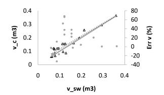
*Fig. 11:* Scattering between the milled volume ( $v_sw$ ) and the calculated volume ( $v_c$ ) of pieces per log and its accuracy (*Err v*)
