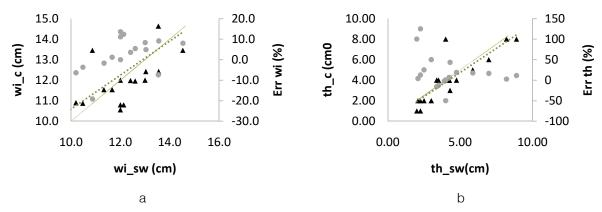
*Fig. 8:* a) Scattering between the width of the piece (*wi\_c*) and the average width of the milled piece (*wi\_sw*); b) the piece thickness (*th\_sw*) and the average milled piece thickness (*th\_c*), and its accuracy (*Err wi and Err th*). Note: c (calculate), sw (sawed), wi (width), th (thickness), Err (Error)
