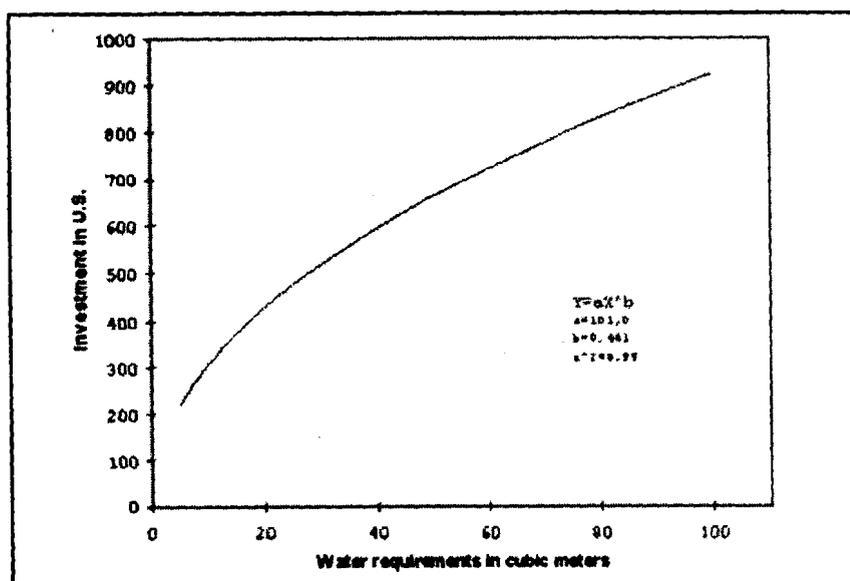
Figure 1: Needed investment for cistern construction as a function of total water requirements
