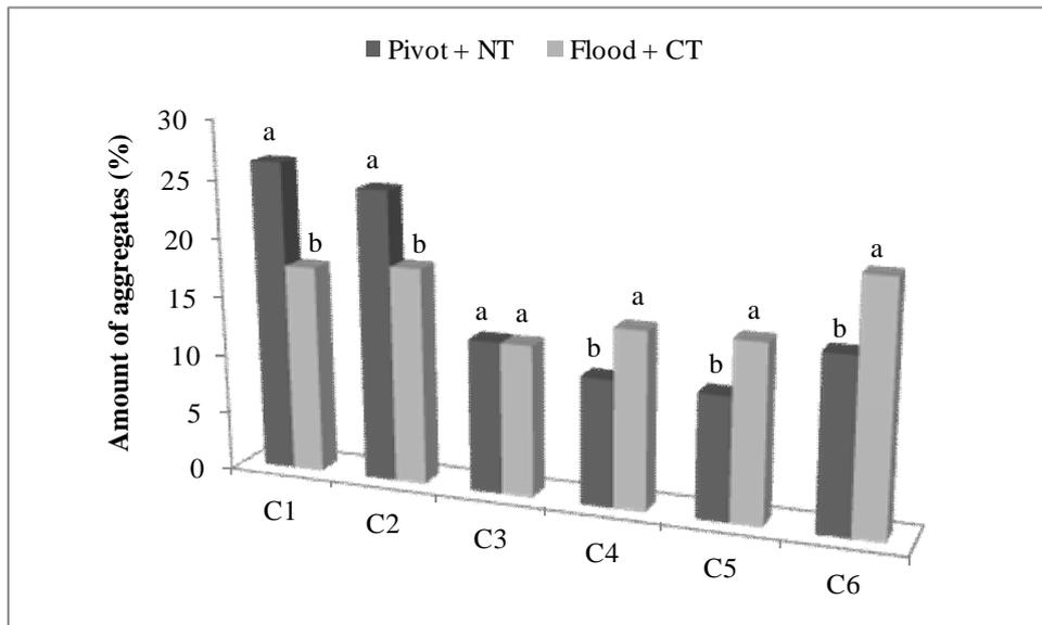
Figure 3 ó Mean values of six aggregate size distribution classes obtained by wet sieving from two rice irrigation and cultivation systems: sprinkler with no tillage (Pivot + NT) and flood with conventional tillage (Flood + CT), where C1 (9.52 ó 4.76 mm), C2 (4.76 ó 2.00 mm), C3 (2.00 ó 1.00 mm), C4 (1.00 ó 0.50 mm), C5 (0.50-0.25) and C6 (<0.25). Different letters represent significant difference between mean values (Mann-Whitney test,  $p < 0.05$ ).
