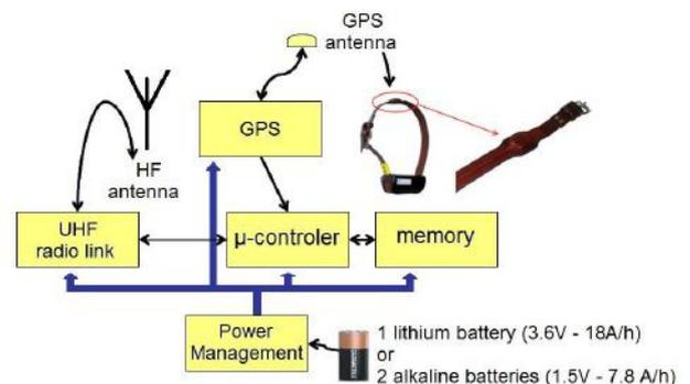
Fig. 3. General architecture of the electronic collars [9].
