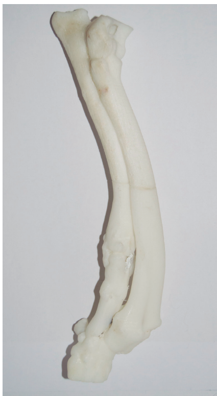
Fig.4. Printed 3D model in ABS, using a FDM printer, of the right forelimb antebrachium of the dog, lateral view.
