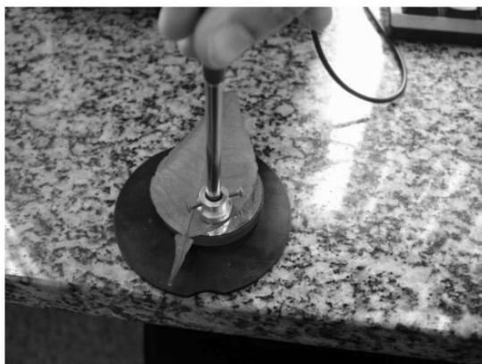
**Figure 2.** All measurements were performed with the leaves *in natura* positioning the optical fiber probe perpendicularly on its ventral portion near the midrib, taking care that light does not focus directly on the veins of the leaf.
