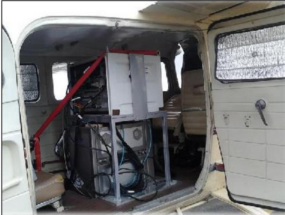
Figura 5 – Sensor LIDAR Aerotransportado Harrier 68i instalado na aeronave Cessna-206.
