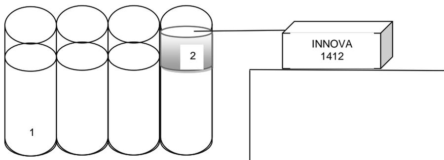
1. Composting reactor; 2. Static chamber.
