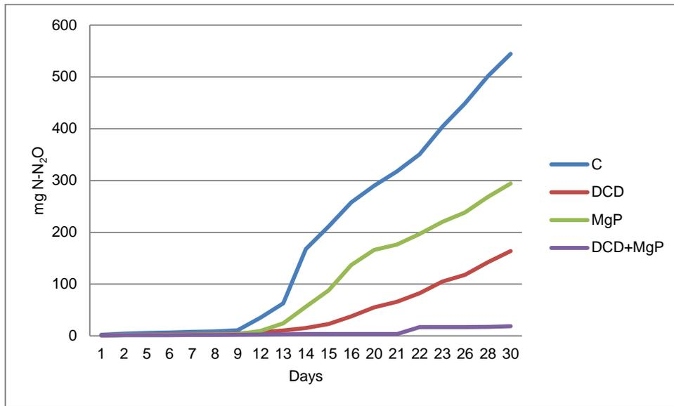
**Figure 2.** Accumulate emission of N-N<sub>2</sub>O during the experiment.
