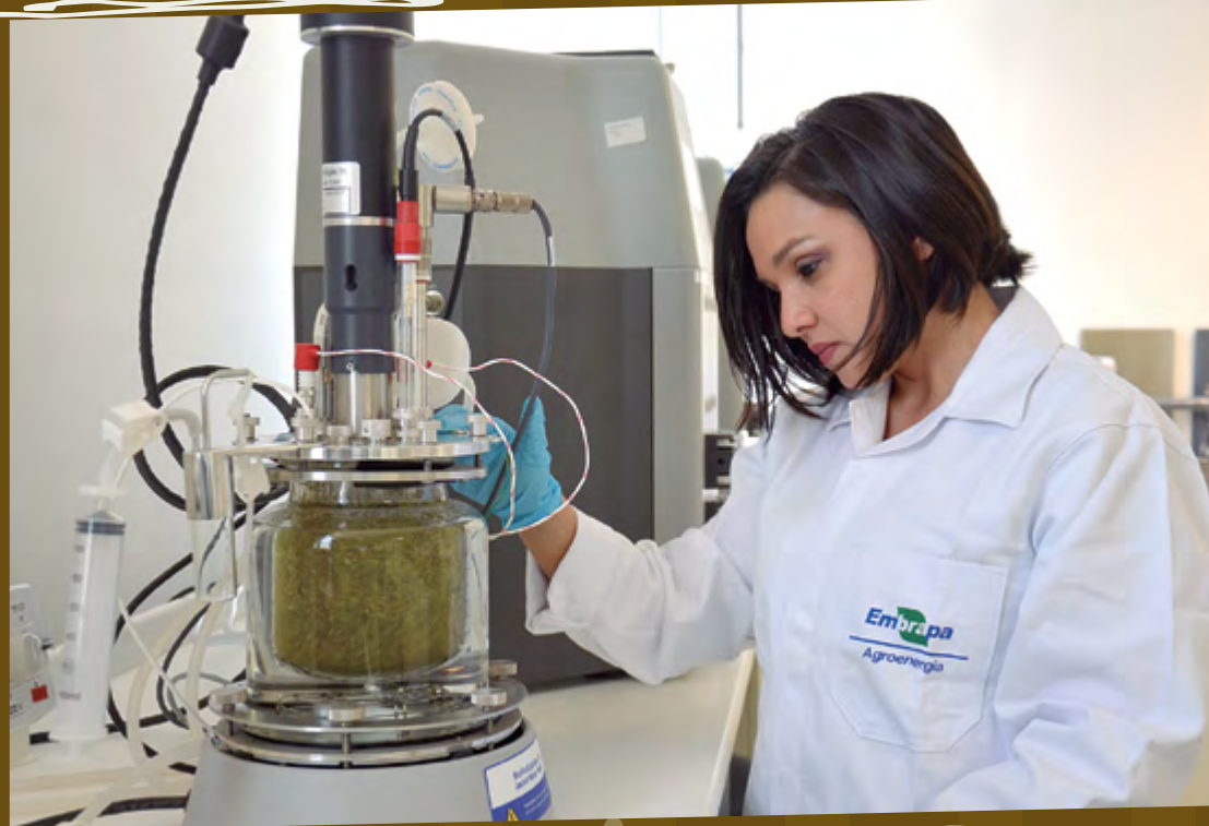
Silvia Belém, from Embrapa Agroenergia, observes a reactor during the production of ethanol from elephant grass
